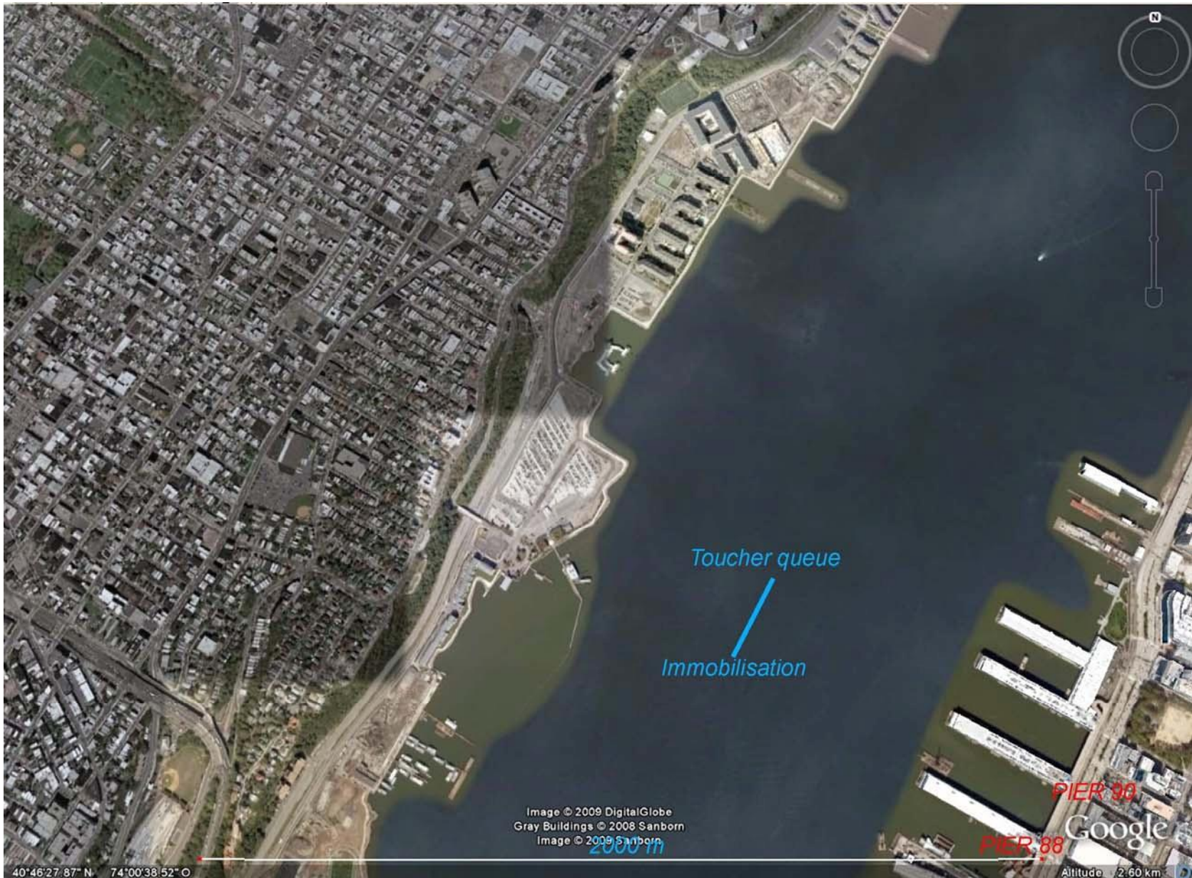
Figure 1. Touchdown location based on BEA analysis of video footage of the water landing. “Toucher queue” is the touchdown point, and “immobilization” is the point where the airplane came to rest relative to the water.
